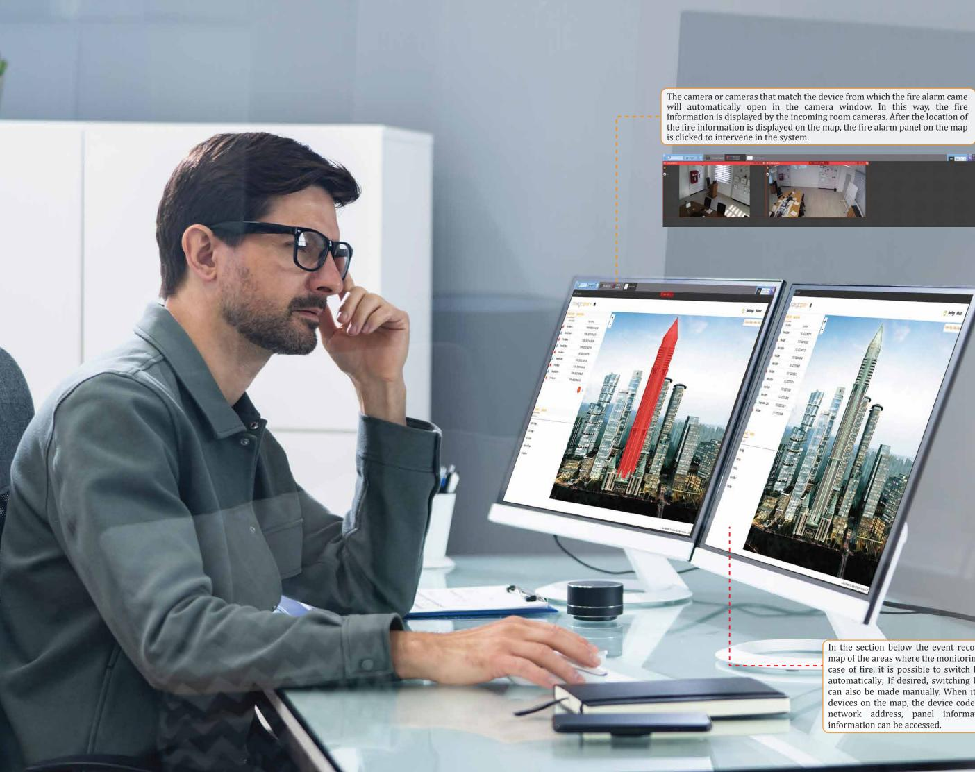
In the section below the event records, there is a map of the areas where the monitoring was done. In case of fire, it is possible to switch between maps automatically; If desired, switching between maps can also be made manually. When it comes to the devices on the map, the device code, device name, network address, panel information, address
